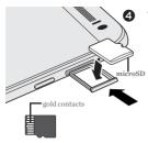
4. With both the phone and the microSD tray facing up, place your microSD card into the tray, with the gold contacts facing down and the narrow side facing in.
