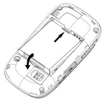
3. Line the battery cover up correctly and push gently to close.
