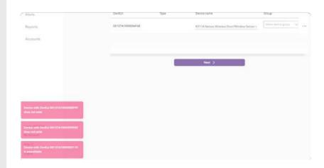
Note: Efento devices limit the number of transmissions to optimize the battery lifetime. By default, the devices will log a reading every 5 minutes, and upload all those readings every 3 hours. You can configure the device Edge Rule to trigger **real time alerts** if certain conditions are met.
